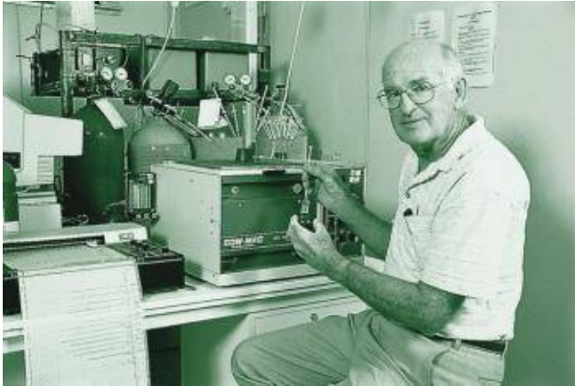
Figure 1. Barry McGlasson, University of Western Sydney Hawkesbury, Richmond Campus, using a gas chromatograph (fitted with a flame ionisation detector) to analyse ethylene concentrations in samples of air exiting enclosed containers of harvested fruit.
