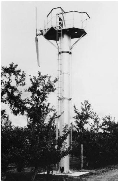
Figure 14.26 Alleviation of frost damage with wind machines. During a temperature inversion, upper air layers are warmer than the air at tree level, and these huge fans can be used to drive the warmer air down into the trees and across the ground to counter radiative heat loss. A special variant has involved use of helicopters as mobile adjustable fans. Operating costs are much higher and maintaining a low-flying circuit in pre-dawn darkness can be hazardous! (Photograph courtesy E.W. Hewett)
