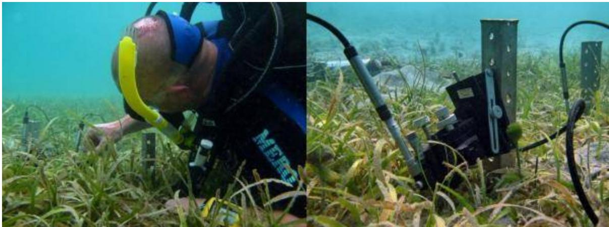
Figure 1. Diver operating O<sub>2</sub> and H<sub>2</sub>S microelectrodes (left) in a *Thalassia seagrass* meadow in the Caribbean. Development of *in situ* equipment has enabled measurements of internal aeration under challenging field conditions in aquatic systems (right). (Photographs courtesy of Malene Hedegård Petersen (left) and Ole Pedersen (right)).
