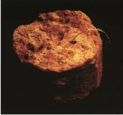
Figure 3.42 Sample of dense subsoil containing a biopore occupied by a root. Such biopores are passages for roots through otherwise almost impenetrably dense soil.
